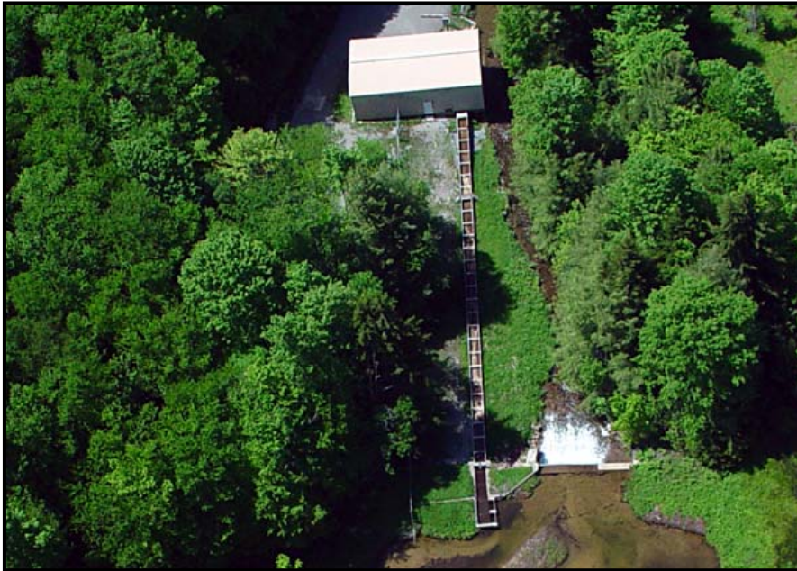
Figure 3-25: A limestone treatment system in the upper reach of Otter Creek. The system is designed to regulate the addition of crushed limestone to the stream to maintain pH levels in a range suitable for fish. Without treatment, most of Otter Creek would be too acidic to support fish.
